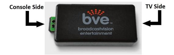
The dynamic Broadcastvision Entertainment AXSCAB accommodates many varied applications to allow console control of Personal Viewing Screens and to facilitate operation of cable/satellite/IPTV set top boxes (STB). The CAB product should operate in a "plug-and-play" manner. Just note the side labeled TV above and connect appropriately with the cable provided.
