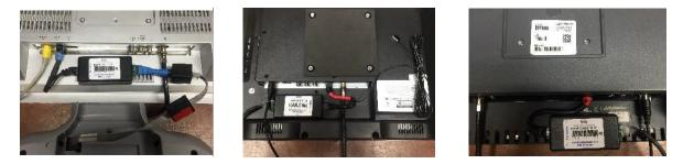
**Note:** On newer Precor 15" screens the CAB will not fit behind the plastic shroud. Because of this a 2' flat cable extension is included with these Precor CAB's to allow you to mount the CAB on the back of or inside the Precor console.
