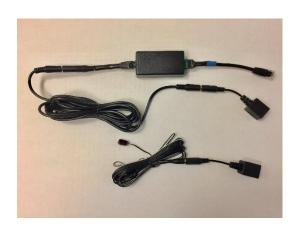
5. After the IR cable has been run through the machine the IR emitter should be placed over the infrared eye on the front of the set top box. If you cannot see where the IR eye is on the front of the STB, shining a flashlight at the front of the box will usually help you to see the IR eye. Please see the IR eye locations of some of the most common STB's below:
